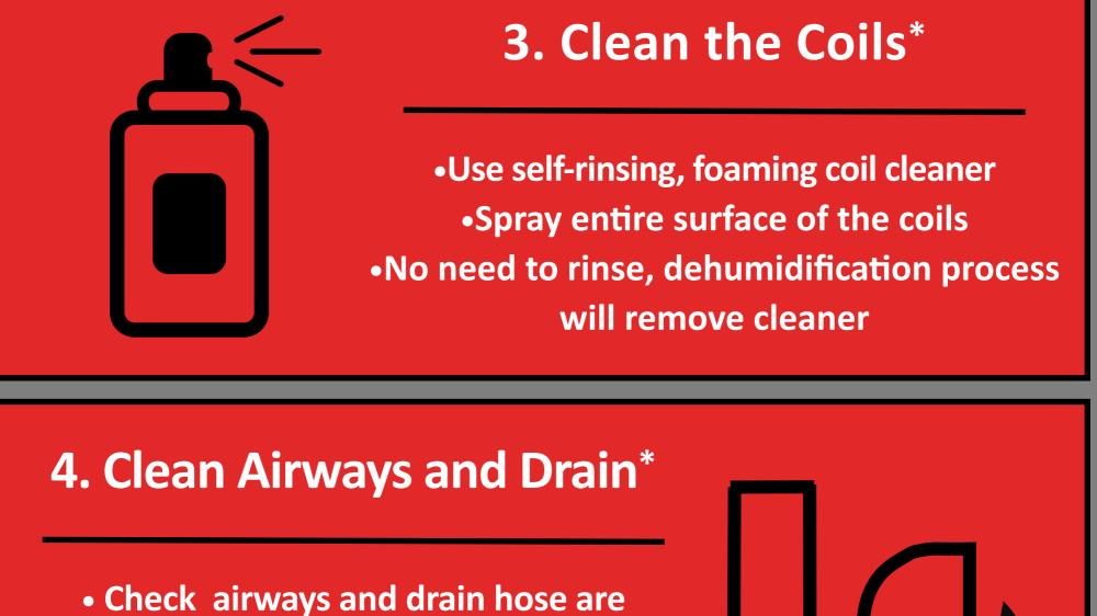
unblocked and connected Make sure collected condensate can flow continuously
