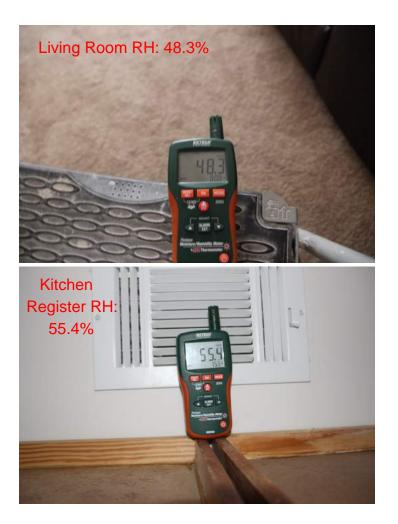
Problem solved? Yes. We performed fungal IAQ (Indoor Air Quality) testing at installation and a week later, with two 600 CFM HEPA scrubbers and a 200 CFM unit operating in the apartment with a second hydroxyl ion unit during that week.
